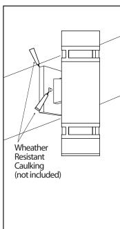
After Installation, seal around the top and side perimeter between the fixture and the wall surface with weather resistant caulking. The bottom should be left un-caulked to prevent moisture build-up. Apply a small amount of weather resistant caulking around the side perimeter between the cap nut and mounting plate.
