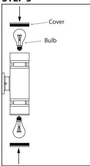
Install specified bulb type and wattage (not included). Push covers onto the fixture.
