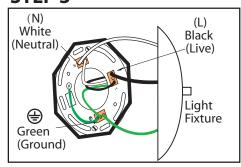
Connect (push) electrical wires from fixture into correct inserts. Black (live), White (neutral), Green (ground)
