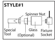
**Style#1** - Remove spinner nut from the socket. Place the glass onto the fixture socket. Use the special tool that comes with your fixture to tighten the spinner nut onto the socket to secure the glass in place.
