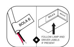
ONE AT A TIME, WIRE LAMPS TO MATCHING DRIVERS. CUT EXCESS WIRES IF NECESSARY
