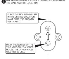
USE THE MOUNTING PLATE AS A TEMPLATE FOR MARKING
