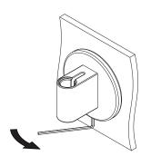
PROUTE THE POWER CABLE UP THROUGH THE HOLE AND PLUG INTO LAMP BEFORE INSERTING THE LAMP INTO THE MOUNT.
