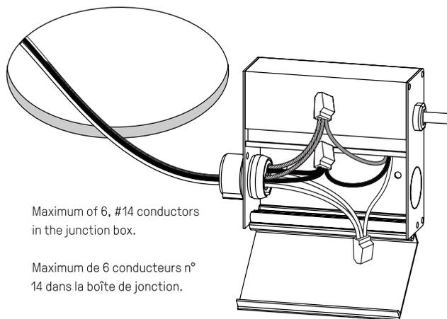
Maximum of 6, #14 conductors in the junction box.
